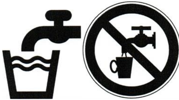
Figure 6 - Signs "Potable water" (left) and "Non-potable water" (right) according to EN 806-2
